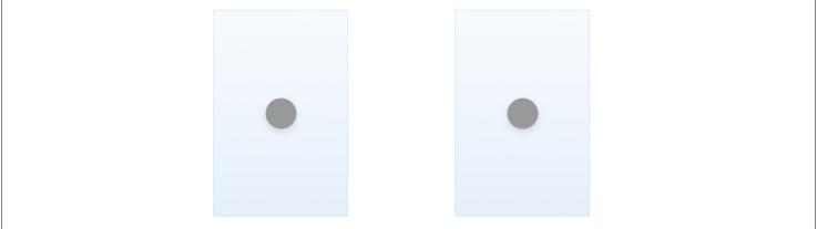
Example 2: Side-by-side V-H Pol, Recommended orientation for enhanced MIMO performance with horizontal separation of 0.8" or greater for optimal isolation
