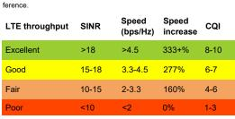
The LTE radio automatically selects the best throughput based on measured SINR.
