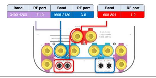
Note: The RET Device for 3400-4200 MHz is connected via the 1695-2180 Port 3 Bias T port or 1695-2180/3400-4200 MHz AISG ports.
