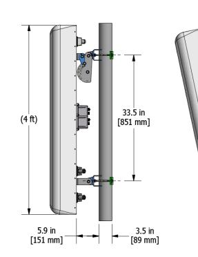
CSS P/N: 919011 BRACKET KIT 2 POINT, 12 DEGREE DOWN TILT SHOWN MOUNTED ON 3.5" O.D. POLE 3.5" O.D. MAX POLE SIZE
