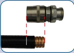
Align center conductor as shown with end of cap. Mark cable jacket (using pen or marker) in line with end of connector.
