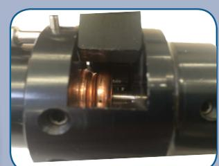
Make sure blade is positioned over valley closest to end of cable, release blade lever and actuate drill until cable is completely cut.
