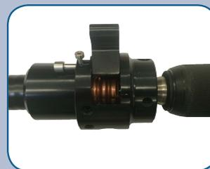
Actuate drill until outer conductor reaches fixed stop; this will remove jacket.
