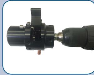
Hold drill and pull stripping tool forward to eject the cable slug. Make sure any remaining cable is removed from tool.
