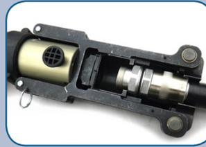
Pull/push back the insert to allow connector/cable to lay flat in frame. Make sure connector is fully seated.
