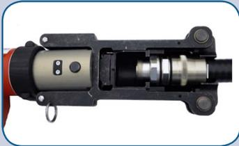
Press HCG tool trigger until gun cycles. Do not pull or push on tool or cable during compression.
