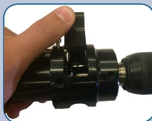
Attach prep/strip tool to drill. Open blade lever and lock with pin. Insert cable and actuate drill.
