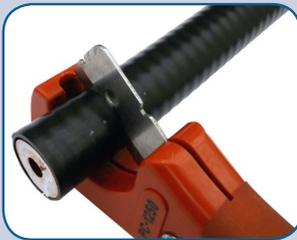
Straighten cable and position RDCUTTER-S in valley of corrugation and cut off cable squarely.
