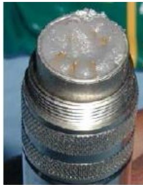
Fig. 7 – Proper Dielectric Grease Application
